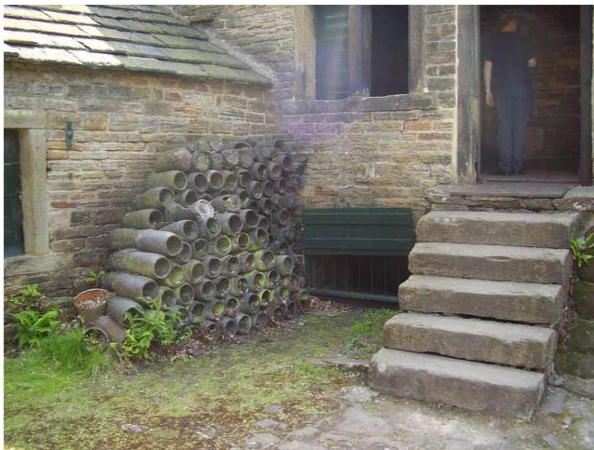
Crucibles for quality steel melting. Early 19th century.
