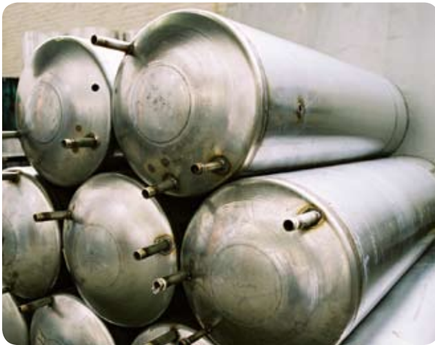
Stamped top and bottom of boilers, in grade 441, S. Africa.
