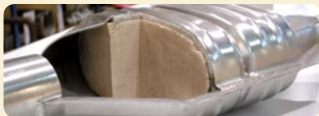
Stamped catalytic converter housing, in grade 441.
