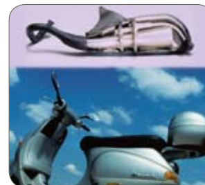
Grade 1.4509/441, Centro Inox, Italy. The new Vespa ET2 is equipped with a ferritic catalytic silencer.
