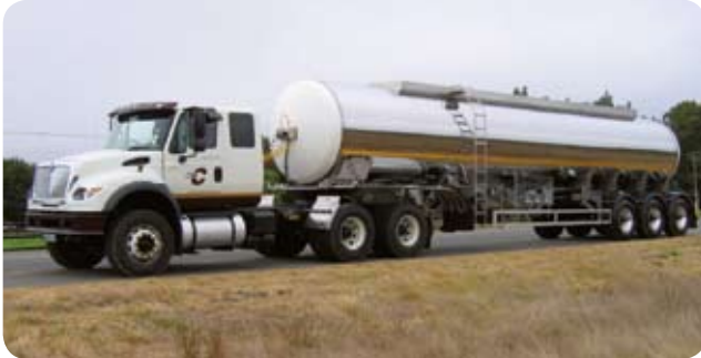
Milk tanker, cladding in grade 430, S. Africa.
