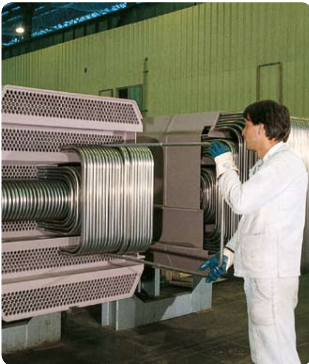
Moisture separator reheater in grade 439, Europe.
