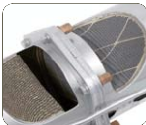
Grade 1.4509/441, diesel particle filter, Peugeot 607, Faurecia
